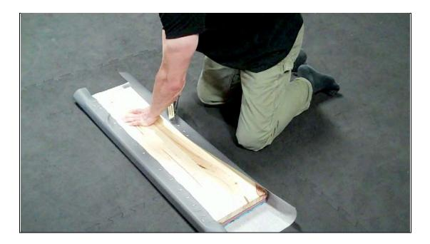
One length-side has been attached and working now on the opposite side. Make sure to keep plenty of tension on the vinyl as you staple it into place.
