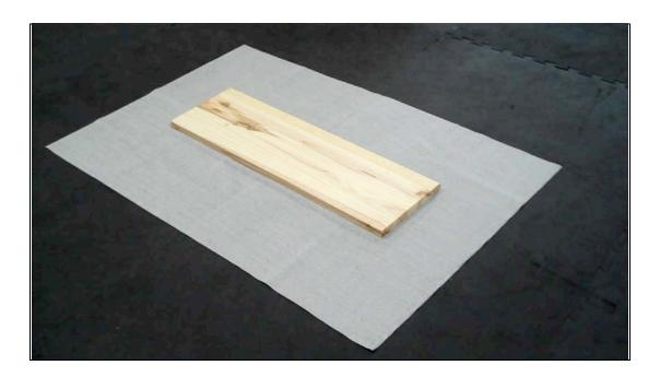
This is step one, laying out your vinyl with the board placed on top of it. Notice that the smooth side of the vinyl is towards the floor.
