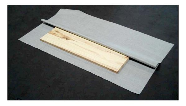
Here we do the same thing with the other side of the vinyl. The fold that you see on the upper portion is where the vinyl will be cut with the scissors.
