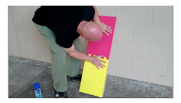
This is all so easy to do. I take the foam section and slap it onto the board which is sticky from the adhesive. The key here is to make sure that you keep the sides of the foam completely even with the edges of the board. If you're off a little bit, just pull the foam off, line it back up and place it back on.
