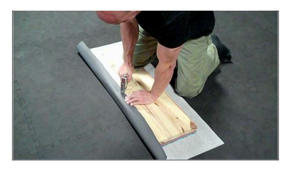
This is the most technical phase of the entire project; all you have to do now is operate a staple gun. So load it up and let's go... Take the board and place it so that the foam pieces are in contact with the underside of the vinyl. Make sure that the board is centered on all four sides and you're ready to staple.
