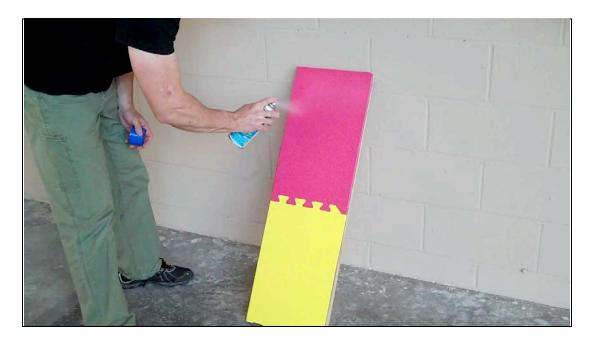
With the first layer of foam in place, this first foam section gets a coat of adhesive to prepare it for the next layer of foam. *Reminder:* Do this in a well-ventilated area.
