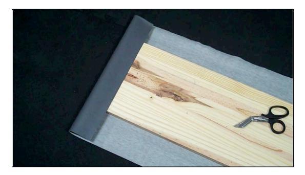
As before, I have placed the board where I want the vinyl to overlap on one end so that I will only have to cut once on the other end. So far I have not used either a ruler or tape measure for any of this. I just used the width of my four fingers as a rough measure for all four sides of the board.
