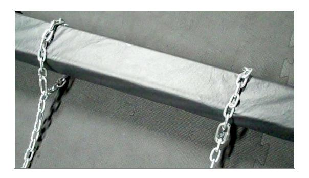
Below is a close-up view of the screw-tight chain links after they have been slipped through the end links of the chain. Our last step is to wrap these chains around a suitable overhead support. Depending on where you are, this support could be a piece of outdoor playground equipment, a chin-up bar, a tree branch or one of the rafters in your garage or basement.
