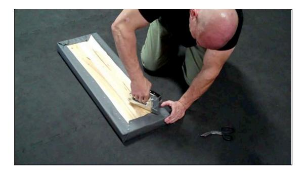
Almost done. The scissors is nearby because I had a spot where the material gathered up to the point it looked too thick to for the staple to attach securely. So I cut a small piece out with the scissors and got it under control.
