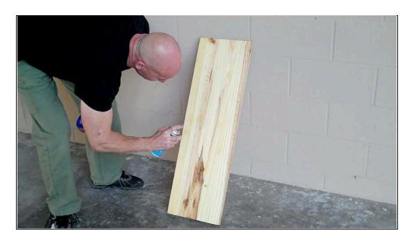
Here I am applying spray adhesive to the surface of the board in preparation to attach the first section of foam.
