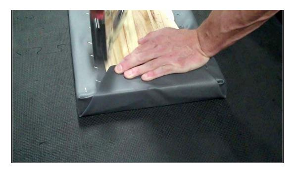
Here's a close-up view of how to handle the ends. It's kind of like gift-wrapping a package. Again, pull tight on the vinyl and use plenty of staples.
