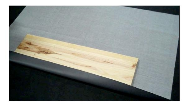
Here you will notice that I slid the board over to one side of the vinyl piece. I then folded the vinyl over what will become the underside of the board. When deciding how much overlap you want, don't forget that the padding you attach to the other side of the board will 'take away' some of the material. It's important that you leave enough vinyl to attach (staple) to the board.
